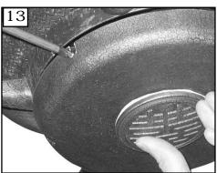
Remove switch housing cap by removing 1 screw without key slots and loosening the other 2 screws and twist to remove.
